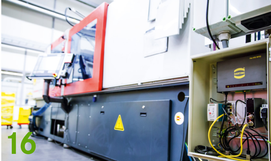
Existing production equipment retrofitted with MICA®
