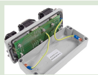
All LED lights have been equipped with cables, flexible protective tubing and 3A HPR connectors.
