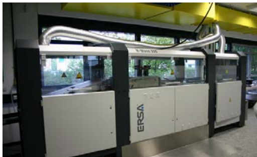
Wave soldering plant
