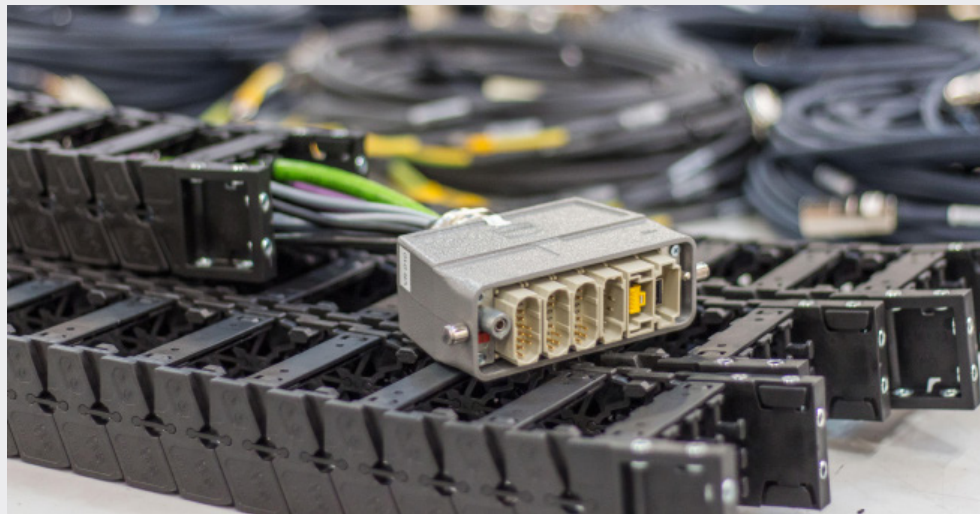
Han® High Density module (three), Han® EE module, Han® RJ45 module, Han® USB 2.0 module (Male variants in each case)
