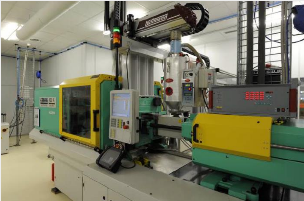
Figure 6: Injection molding machines for producing the MID base substrates
