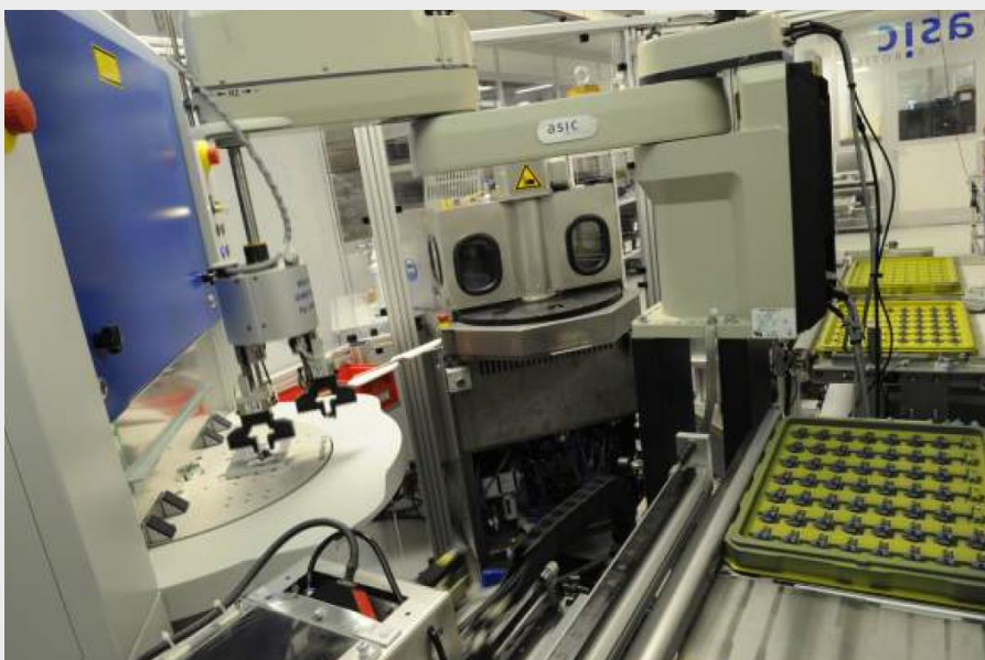
Figure 3: Laser system for structuring substrates with subsequent cleaning.
