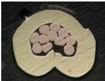
Figure V-7: Cross-section of a defective sample, wire cross-section too small
