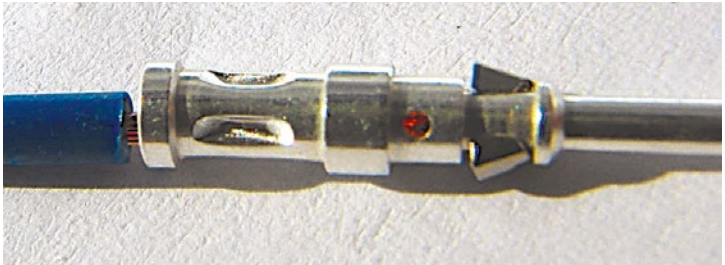
Figure V-12: Turned Han D ® contact - proper stripping (depth + length) - inspection hole filled - crimping is uniformly central
