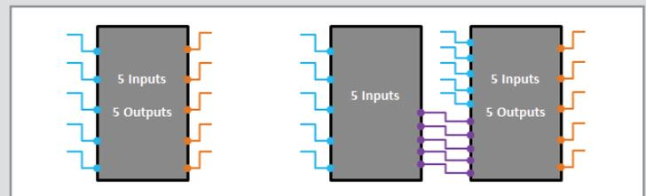
Sketch Displaying How I/O Is Structured in Daisy Chaining Chassis Systems
