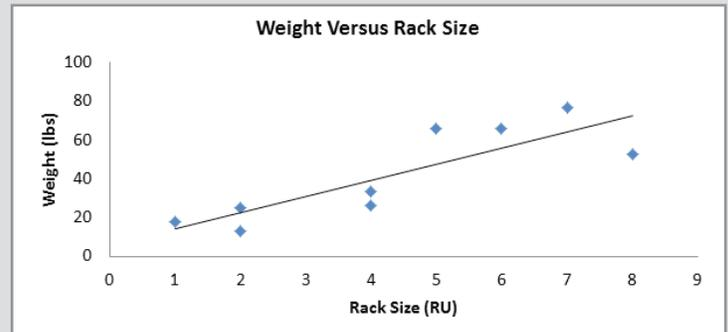
Trend between Weight of Rack Mounted Chassis and Size in RU
