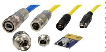
SPE connector variants according to IEC 63171-6: as IP65/67 as well as IP20 versions (upper row from left to right: M12 PushPull, M8 Push-Pull, M8 SnapIn and IP20 connectors / upper row from left to right: M12 socket with screw and PushPull interlocks, M8 socket with SnapIn and PushPull interlocks, angled IP20 PCB socket)
