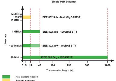
Graphic display of range and transmission speeds for the current IEEE 802.3 SPE standards
