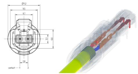
Symmetrical design of the mating face according to IEC 63171-6
