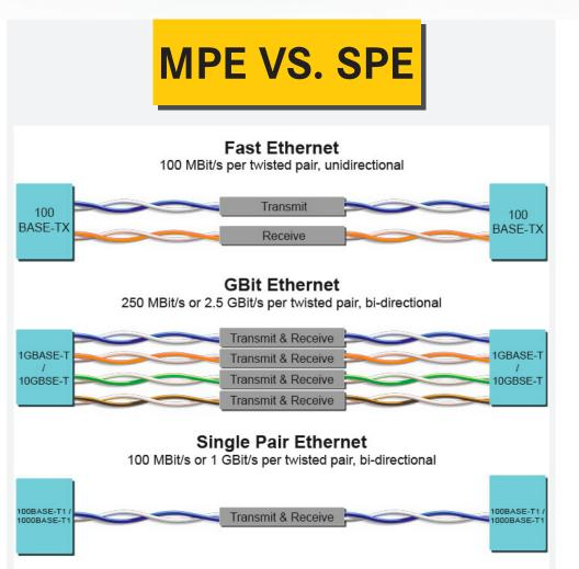
MPE stands for Multi Pair Ethernet, which uses two or four wire pairs
