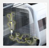
WLAN on-board networks in trains require stable and interference-free networks, and this can be realized with fiber optic connections. These are very sensitive to soiling or even damage when the connection is disconnected and mated. With the help of HARTING lens modules, in combination with the Han-Modular® connector series, an insensitive and protected fiber optic plug connection can be realized
