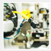
Mini PushPull is the perfect IP65/IP67 housing for the HARTING ix industrial<sup>®</sup>. It combines the well-known advantages of HARTING's PushPull technology with the robust miniaturised Ethernet interface according to IEC 61076-3-124. The capabilities of the HARTING Mini PushPull ix industrial<sup>®</sup> interface are highlighted in industrial Ethernet (type A) as well as in signals and serial BUS systems (type B).
