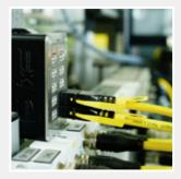
HARTING ix Industrial®: the miniaturised interface according to IEC 61076-3-124. The perfect solution when minimal installation space is available in Industrial Ethernet (type A) as well as for signals and serial BUS systems (type B). A 70% smaller device socket compared to the familiar RJ45: This saves valuable space in the device. The new angled cable connector now saves even more space outside the device.
