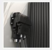
More and more applications on Rail Vehicles communicate via Ethernet connections and existing ones require higher transmission rates. The new Han-Modular® Gigabit Module Cat.  $7_A/8.2$  transmits data in and between the carriages without interference.
